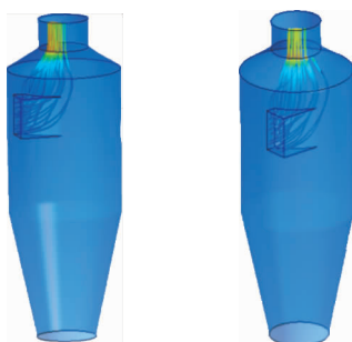
(a) 筒顶角度45° (b) 筒顶角度30°
