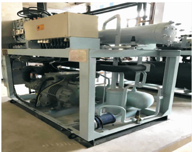
图 1 船用超低温 R404A 单机双级压缩制冷系统试验台部分实物图 Figure 1 Part physical drawing of the marine ultra-low temperature R404A single stage two-stage compression refrigeration system
