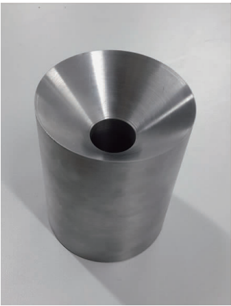
图 3 开式压缩试验装置可更换式内腔套 Figure 3 The sleeve of compression equipment with open mold
