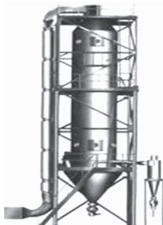
图 1 YPG-22500 压力喷雾豆粉干燥机壳体示意图 Figure 1 Schematic diagram of YPG-22500 pressure spray drying powder casing
